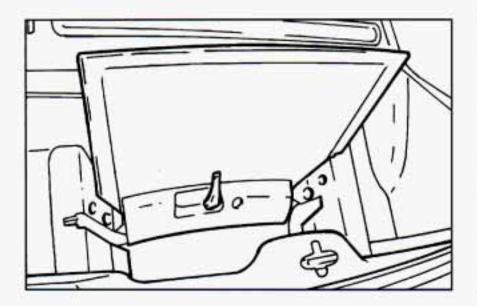
Open the close-out panel completely. Place the panel in the correct slot (driver's or passenger's) in the rear area of your vehicle. Make sure the handle is open and facing you when you put it in the storage slot.
