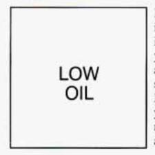
If the LOW OIL light on the instrument panel comes on, it means you need to check your engine oil level right away. For more information, see "Low Oil Light" in the Index. You should check your engine oil level regularly; this is an added reminder.
