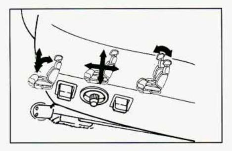
The driver's seat has three controls on the left side.
