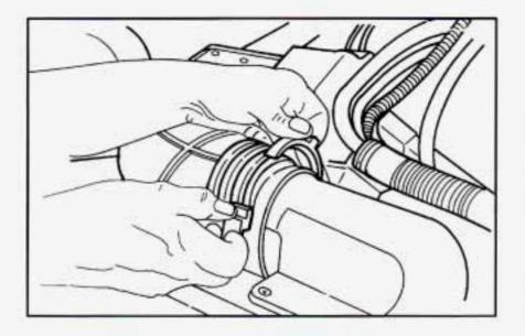
Disconnect the plastic clamp on the duct. Pull apart the connection.
