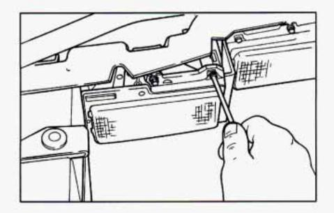
Remove the Torx<sup>®</sup> head screws at the end of the aiming ring.
