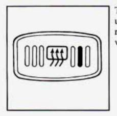
The rear window defogger uses a warming grid to remove fog from the rear window. Do not attach anything like a temporary vehicle license or a decal across the defogger grid on the rear window.
