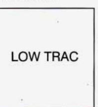
This light will come on when your ASR system is limiting wheel spin. See "Low Traction Light" in the Index. You may feel or hear the system working, but this is normal.
