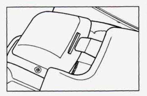
Remove the two side pieces of the boot cover by lifting the rear of cover and sliding them out of their slots.
