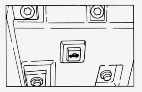
Press the switch in your glove box to unlock the hatch from inside your vehicle. If you have an automatic transmission, your shift lever must be in PARK (P) or NEUTRAL (N) to use the switch. If you have a manual transmission and the ignition switch is in RUN, you must set the parking brake before you can use the switch. The switch only works when the ignition switch is in RUN or ACC, or when RAP is present. (See "Retained Accessory Power" in the Index.)
