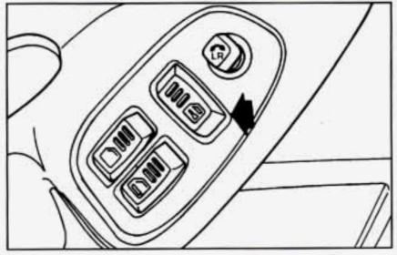
Push the power door lock switch to lock or unlock both doors at once. Note: Operating the power locks may affect the Vehicle and Content Theft-Deterrent/Alarm System (if you have this option). See "Vehicle and Content Theft-Deterrent /Alarm System" in the Index.
