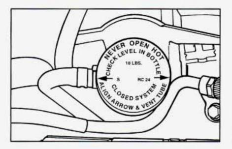
Shut the engine off and replace the pressure cap. Be sure the arrows on the cap line up like this.
