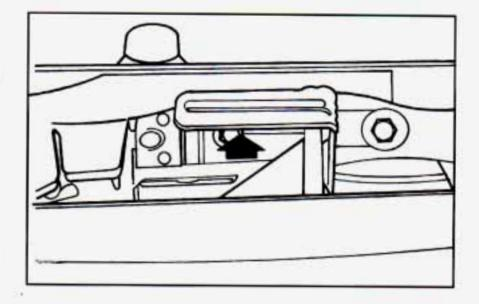
Then go to the front of the vehicle and pull up on the hood release located at the center area of the hood. Lift the hood.
