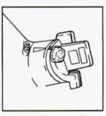
If you have a manual transmission, your ignition lock has a key release button. You must press the button before you can take your key out of the ignition lock.
