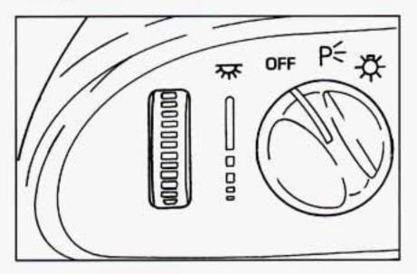
The main lamp control is a knob that works these lamps:
