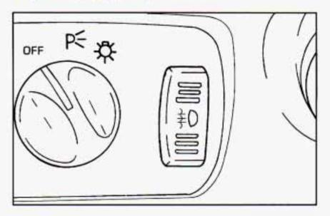
Use your fog lamps for better vision in foggy or misty conditions. Your parking lamps must be on or your fog lamps won't work. D To turn the fog lamps on, push the top of the fog lamp switch. Push the bottom of the switch to turn the fog lamps off. A light on the switch will come on when the fog lamps are on.
