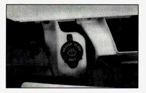
Open the cap labeled WASHER FLUID ONLY. Add washer fluid until the tank is full.
