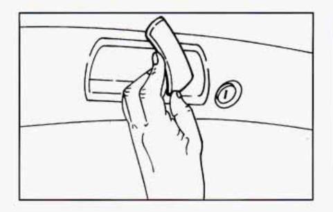
Then pull on the release handle to unlatch the panel. Lift the outer edge of the panel and pull it toward you. Then carry the panel to the rear of the vehicle for storage.
