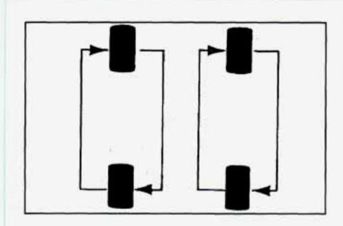
If you have P245/50ZR16 Goodyear Eagle GS-C tires, they must roll in a certain direction for the best overall performance. The direction is shown by an arrow on the sidewall. Because these tires are directional, they should be rotated as shown here. These tires should only be moved from front to rear and rear to front on the same side of the vehicle. Don't include the compact spare tire in your tire rotation.
