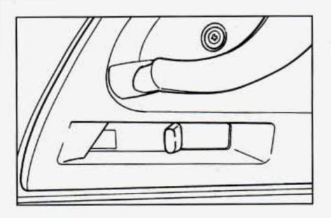
From the inside to lock the door, move the lock control on the door backward.
