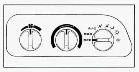
The air conditioning system uses the same controls as the heating system, except that the air control knob has two extra settings, described below.
