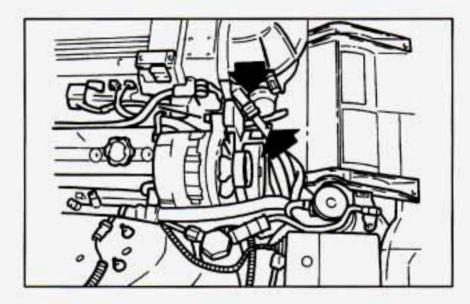
After the engine cools, open the air bleed valves on the heater return hose and water pump inlet.
