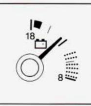
You can read battery voltage on your voltmeter. If it reads less than 11 volts or more than 16 volts while your engine is running, and it stays there, you may have a problem with the electrical charging system.
