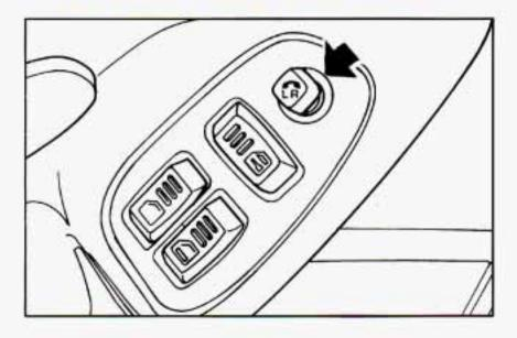
The power mirror control is on the driver's door. To adjust either mirror, turn the switch to left (L) or right (R). Then use the control to adjust the mirror.
