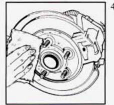
Remove any rust or dirt from the wheel bolts, mounting surfaces and spare wheel.
