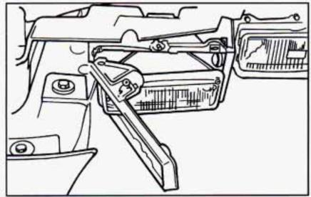
The aiming ring will swing open like a gate. Remove the aiming ring from the assembly. Place it face down, with the aim indicator up. Be careful not to damage the aiming bubble.
