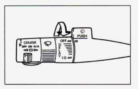
You control the windshield wipers by turning the band with the wiper symbol on it.
