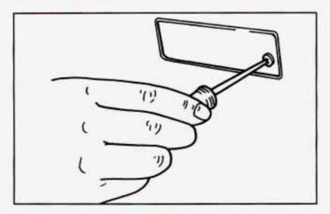
Replacing a rear sidemarker bulb:
