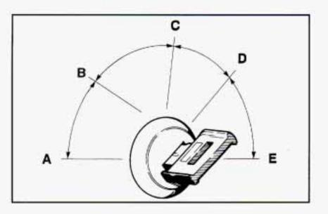
ACC (A): Position in which you can operate your electrical power accessories. Press in the ignition switch as you turn the top of it toward you.
