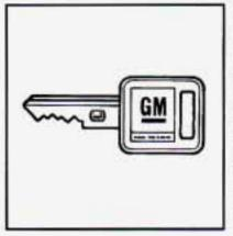
Your vehicle is equipped with the PASS-Key II (Personalized Automotive Security System) theft-deterrent system. PASS-Key II is a passive theft-deterrent system. It works when you insert or remove the key from the ignition.
