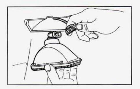
Pull the headlamp out of the assembly. Remove the wiring connector from the headlamp socket by lifting the plastic locking tabs on the connector and pulling it from the socket.
