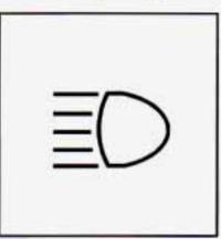
To change the headlamps from low beam to high or high to low, pull the turn signal lever all the way toward you. Then release it. When the high beams are on, this light on the instrument panel also will be on.
