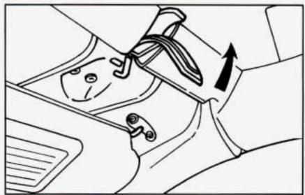
Pull down on the latches and align hooks with holes. Push forward on the larger part of the latch until it clicks. Do not force the latch. If it is hard to lock, the top is not properly aligned.
