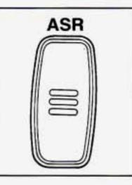
To turn the system off, press the button on the console near the cigarette lighter.
