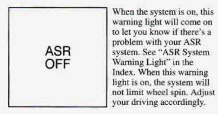
The ASR system automatically comes on whenever you start your vehicle. To limit wheel spin, especially in slippery road conditions, you should always leave the system on. But you can turn the ASR system off if you ever need to. (You should turn the system off if your vehicle ever gets stuck in sand, mud, ice or snow. See "Rocking Your Vehicle" in the Index.)
