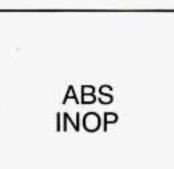
If there's a problem with the anti-lock brake system, this warning light will stay on or flash. See "Anti-Lock Brake System Warning Light" in the Index.
