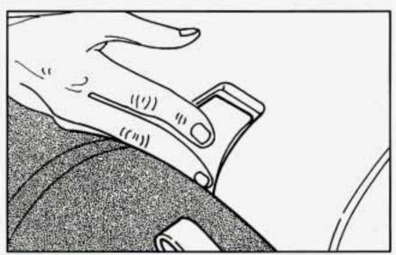
Open the trunk. Remove the middle piece of the cover by pushing in on the latch and lifting up on the cover.
