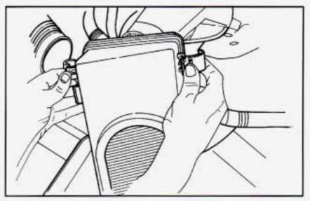
3. Pull the air cleaner straight up. Unclamp the metal clips.
