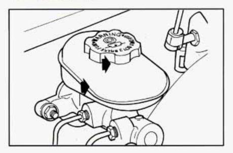
You can check the brake fluid without taking off the cap. Just look at the brake fluid reservoir. The fluid level should be above the plastic seam in the reservoir. If it isn't, have your brake system checked to see if there is a leak.
