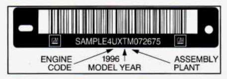
This is the legal identifier for your Chevrolet. It appears on a plate in the front corner of the instrument panel, on the driver's side. You can see it if you look through the windshield from outside your vehicle. The VIN also appears on the Vehicle Certification and Service Parts labels and the certificates of title and registration.
