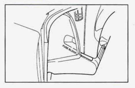
The main fuse block is located on the left side of your instrument panel. Open the cover to expose the fuses.
