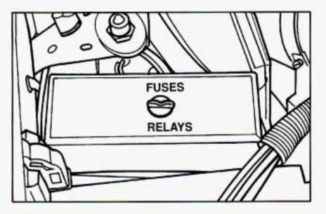
The underhood electrical center fuses are located in the engine compartment. Open the cover to expose the fuses.
