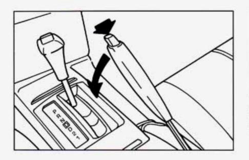
To release the parking brake, hold the brake pedal down. Pull the parking brake lever up until you can push in the release button. Hold the release button in as you move the brake lever all the way down.
