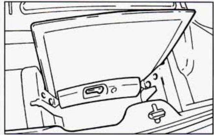
Push the handle closed to secure the panel in the slot. To lock each panel in the storage area, use your door key.
