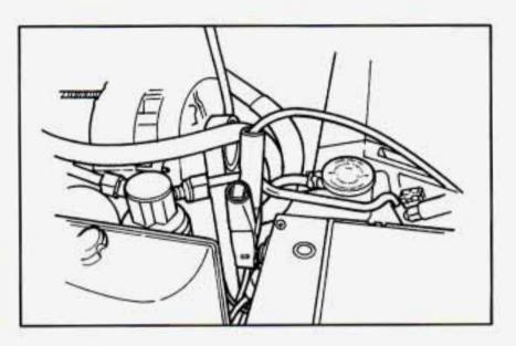
Connect the red positive (+) cable to the positive (+) terminal of the vehicle with the dead battery. Use a remote positive (+) terminal if the vehicle has one.
