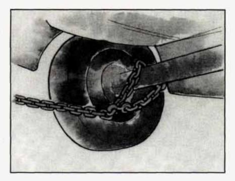
Attach a separate safety chain around each outboard end of the rear axle.
