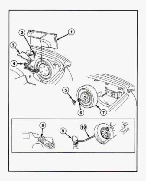
Replace the jack, wheel wrench and flat tire using the storage instructions. When you replace the trim panel, be sure to tuck it under the weatherstrip.
