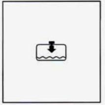
This warning light should come on while you are starting your engine. If the light doesn't come on, have it repaired.
