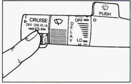
Suppose you set your cruise control at a desired speed and then apply the brake or clutch pedal. This, of course, shuts off the cruise control. But you don't need to reset it. Once you're going about 25 mph (40 km/h) or more, you can move the cruise control switch from ON to R/A (Resume/Accelerate) for about half a second.
